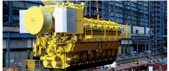
Fig. 1: MAN medium speed four-stroke engine; mainly used in cruise vessels, ferries and large multi-purpose freighters.
