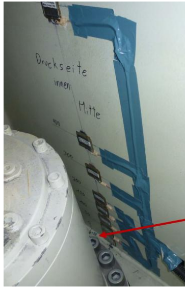
Application of strain gauges on slewing column (and adapter) compression side
