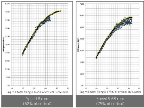
Figure 2 - Rocky power draw (blue diamonds) compared to Morrell C-model prediction (black triangles) as mill fills at
