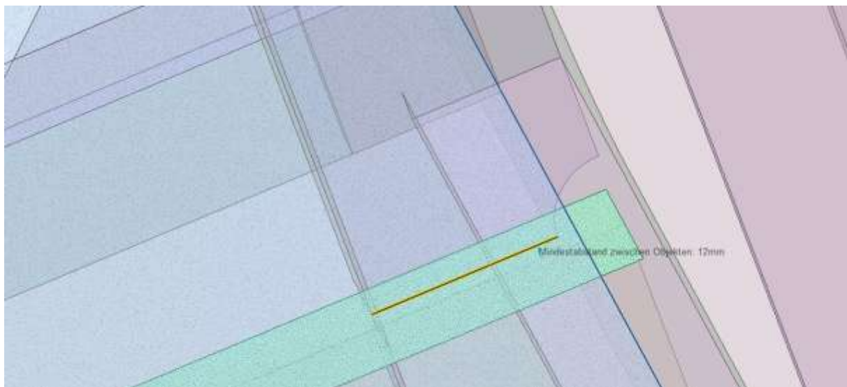
Fig. 11: Gap between T-joint parts
