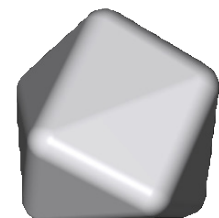
◀ Eight-corner polyhedral particles were used in the simulations
